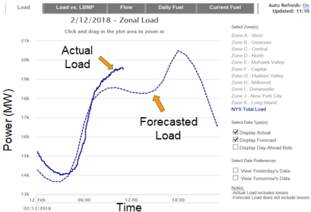
Figure 1.1.2: NYISO Load forecast (dotted) and actual load graph (solid) for 2/12/18. [1]
